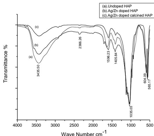
Fig. 2. FTIR Spectrum of HAP powders. (a) Undoped HAP, (b) Zn/Ag doped HAP, (c) Zn/Ag doped calcined HAP.
