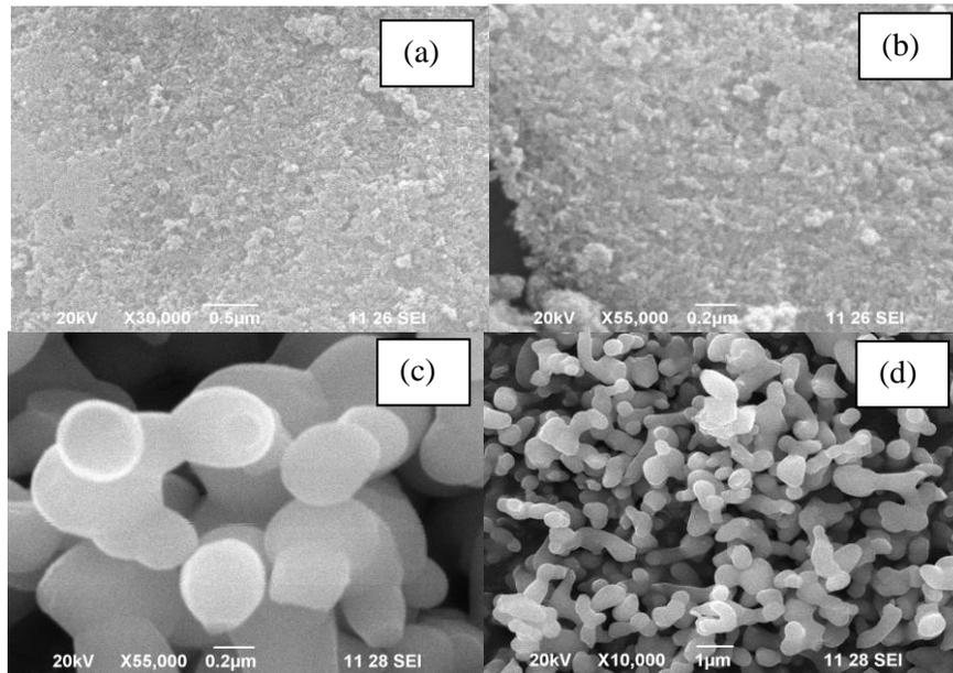
Fig. 3. FE-SEM images of nanosized HAP powders: (a–b) synthesized Ag/Zn doped HAP; (c–d) Ag/Zn doped calcined HAP.
