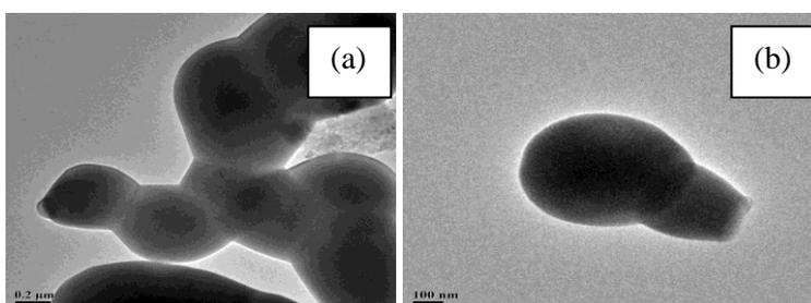
Fig. 5(a-b). FE-TEM images of calcined Ag/Zn doped HAP with spherical rod shape.
