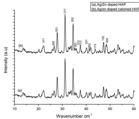
Fig. 1. XRD-analysis of hydroxyapatite powder. (a) Zn/Ag doped HAP; (b) Zn/Ag doped calcined HAP.
