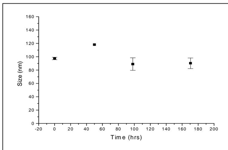
Fig. 1. Liposome size measurements with time during the transfer experiment. Donor liposomes (EiPC/DCP/CHOL (7:1:2)) were loaded with  $^{14}\text{C}$  Chol and mixed with acceptor neutral liposomes (POPC/CHOL (8:2) in a relation (1:10) at 25 °C. In the presence of iso-osmolar sucrose buffer (290 mM sucrose, 10 mM Trizma pre-set crystals and 0.02% Na azide, pH 7.4).
