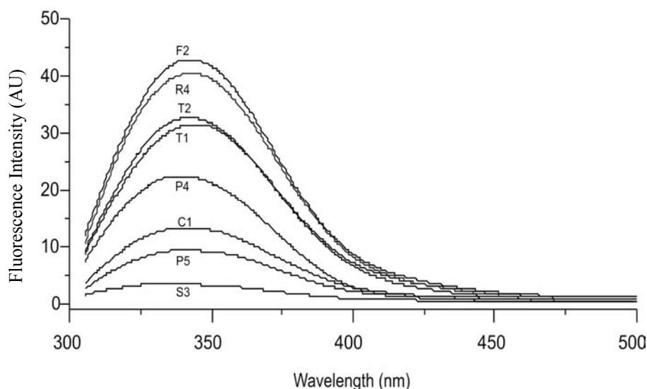
Fig. 4. The emission spectra of the fluorescence for  $\lambda_{\text{ex}} = 295$  nm, in arbitrary units (AU).
