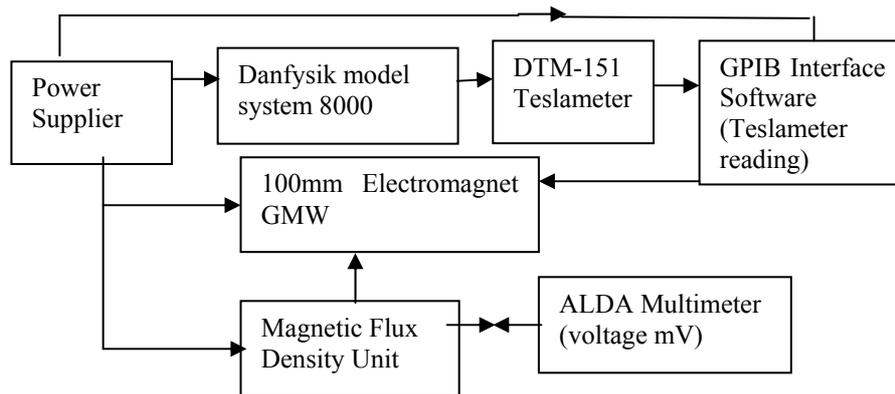
Fig. 1. Schematic diagram illustrating calibration of magnetic flux density unit.
