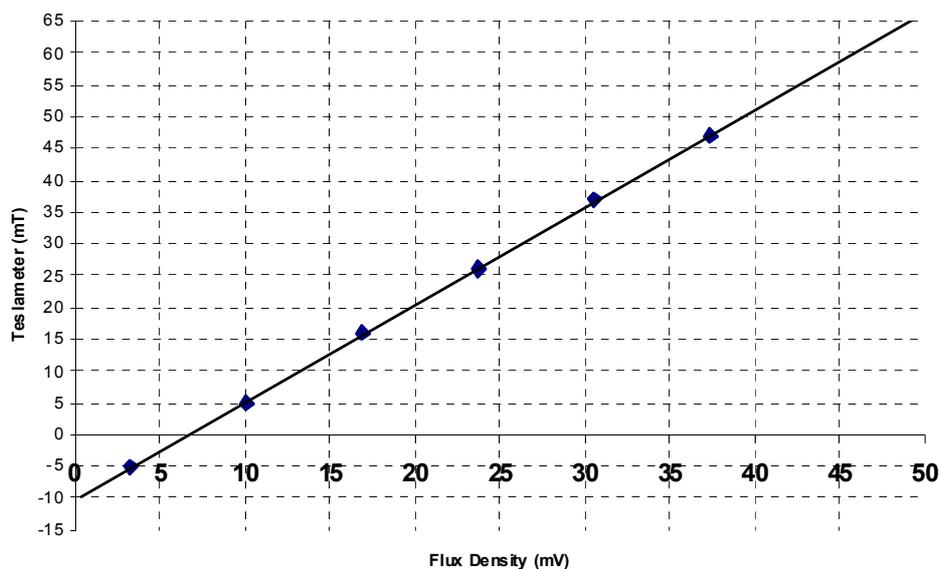
Fig. 2. Flux density versus B-field as per teslameter reading.
