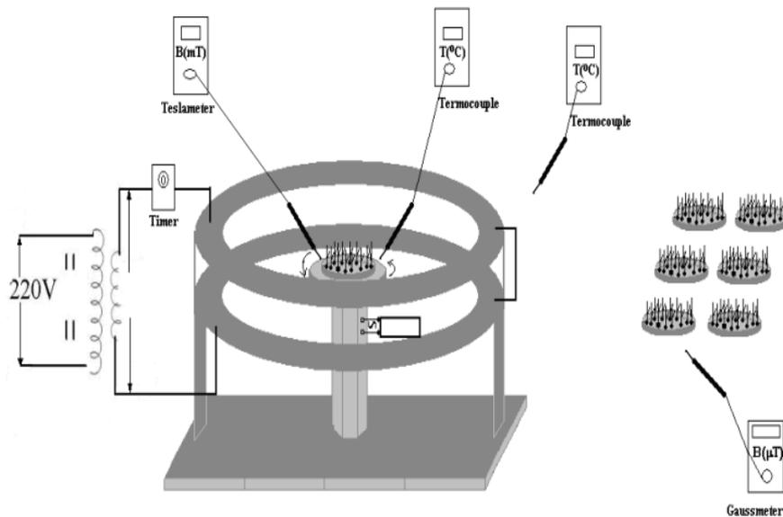
Fig. 1. The schematic representation of the magnetic exposure designs.
