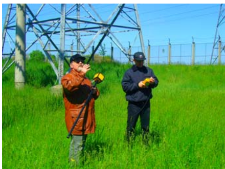
Fig. 7. Measurement of low-frequency electric fields under high voltage power lines.
