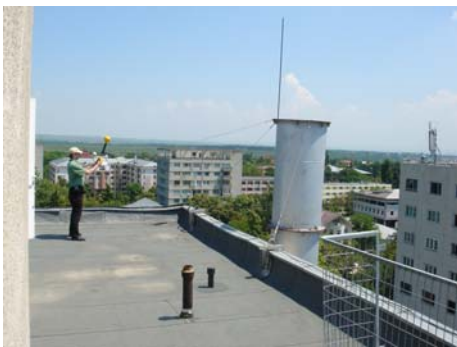
Fig. 5. Measurement of high-frequency radiation emitted by various antennas.
