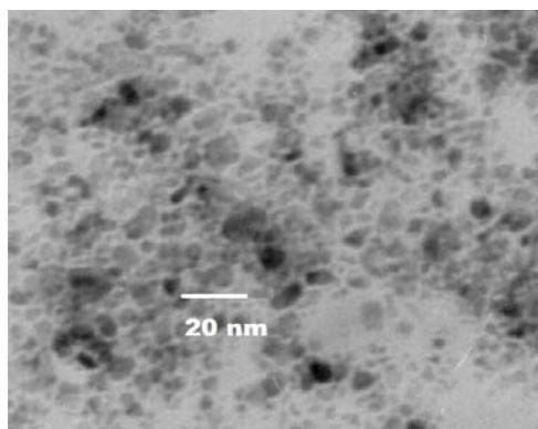
Fig. 2. TEM images of magnetic NPs of  $\text{CoFe}_2\text{O}_4$ .
