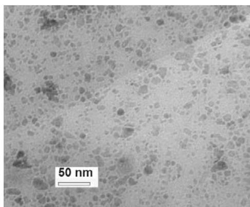
Fig. 1. TEM images of magnetic NPs of  $\text{Fe}_3\text{O}_4$ .
