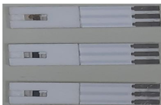
Fig. 4. \text{Na}^+ , \text{Cl}^- and glucose sensors.
