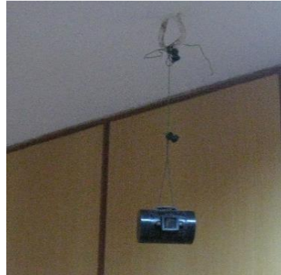
Fig. 7. SSNTD in formica laminated room.
