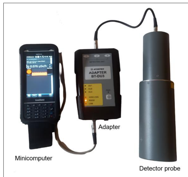
Fig. 2. Photograph of the AT6101C(E) spectrometer used in this study to measure the ambient gamma dose equivalent rate.
