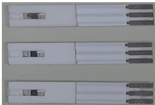
Fig. 4. \text{Na}^+ , \text{Cl}^- and glucose sensors.
