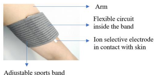
Fig. 8. Wearable sweat monitoring system on arm.
