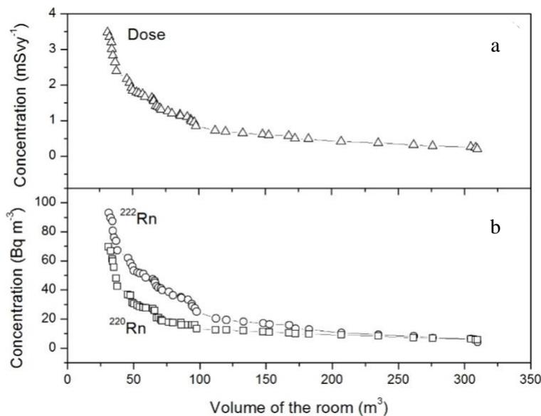
Fig. 1. <sup>222</sup>Rn and <sup>220</sup>Rn concentration variation with the volume of the room.
